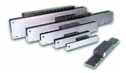
The forcers are ironless, which means that there is no attractive force and no disturbance forces generated between forcer and magnet track. The ironless coil assembly has low mass, allowing for very high acceleration.
